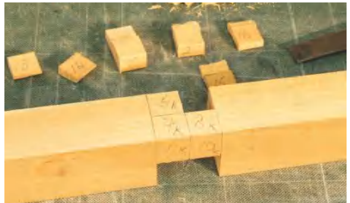
▲ Pic.6 Carefully chop out the squares that you are not keeping
